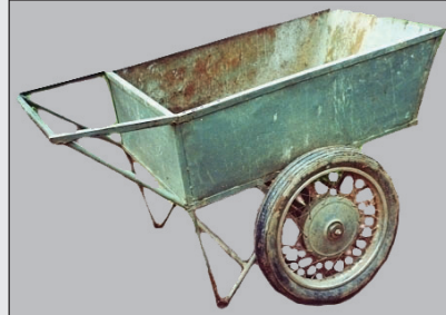
Simple handcart with motorcycle wheels, Lusaka
