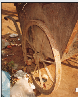
An iron wheel on a handcart in Delhi. The combination of solid wheel and poor bearings would make this a difficult cart to use.
