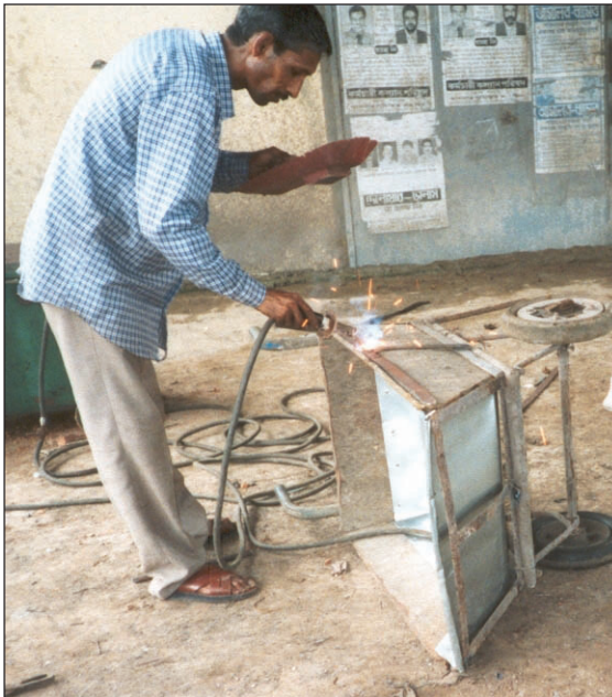
Manufacturing a handcart in Dhaka
